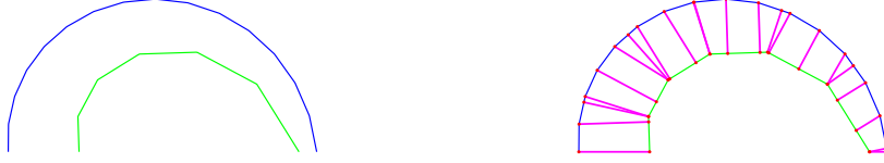
Figure 5.1: Left: Two curves. Right: Their Fréchet morphing. Since the Fréchet morphing computed inside each cell of the free space diagram is a segment, it is enough to mark all the critical configurations when the morphing enters/leaves a cell. Each critical configuration is depicted on the right by a segment connecting the two points being matched. In between two such configurations, the morphing is the linear interpolation between the two configurations. See here for an animation of this specific morphing.
